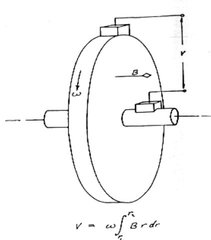
The inertial force on the magnet disk can be held as a constant while increasing the radius and still achieve increased power output as the following analysis will show.
