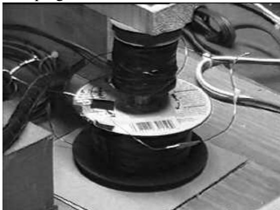
Damping Coil Under Balance Beam Arm
