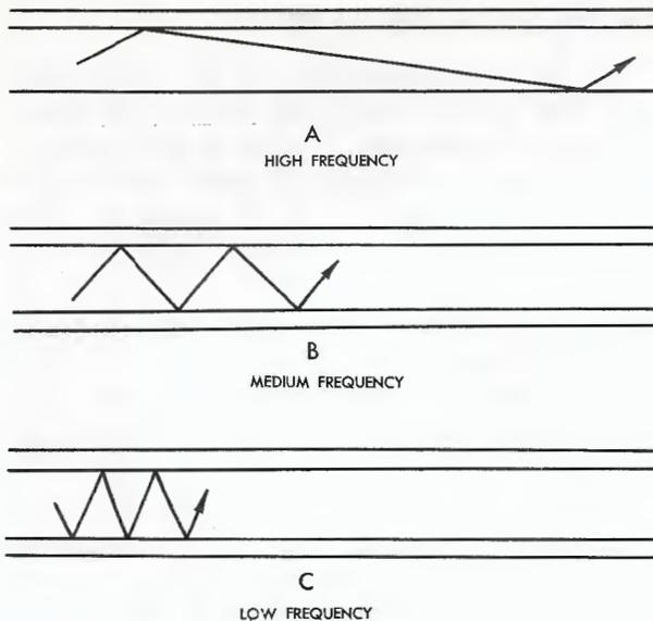
Figure 11-21. Angle at which Fields Cross Waveguide Varies with Frequency
