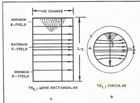
Figure 11-24. How to Count Wavelengths for Numbering Modes
