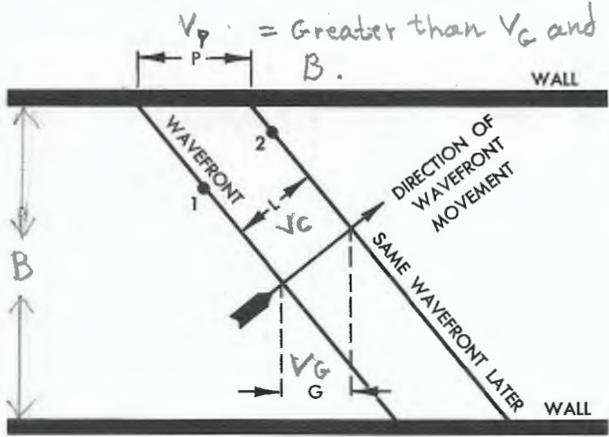
Figure 11-22. Relation of Phase, Group, and Wavefront Velocity
