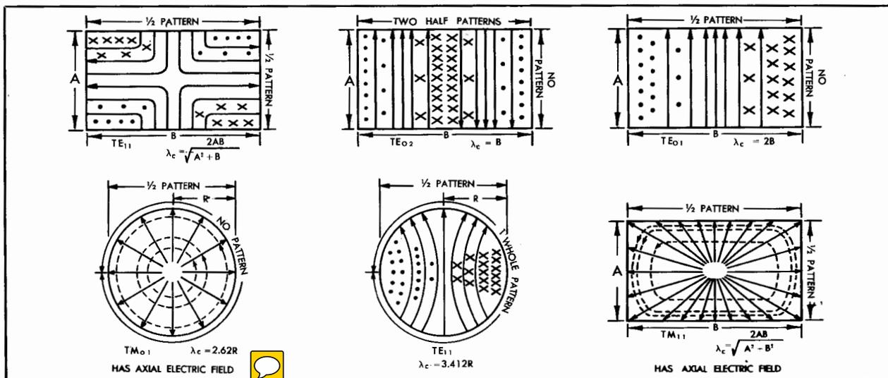
Figure 11-25. Various Modes in Waveguides
