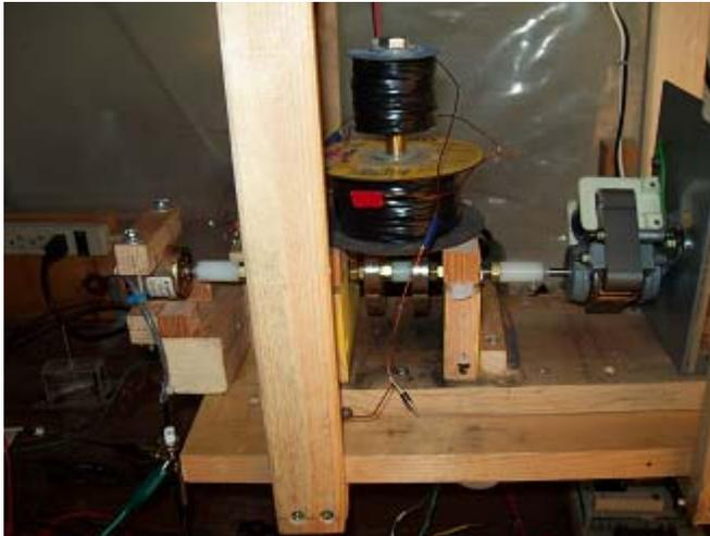
The small motor at the far left is a small permanent magnet d.c. motor which is used as a conventional generator for comparison to the large a.c. pickup coil at the center of the picture. The drive motor is an a.c. 110 volt fan motor from an old microwave. It normally runs at 3600 RPM. This is located at the far right in Fig. 1.
